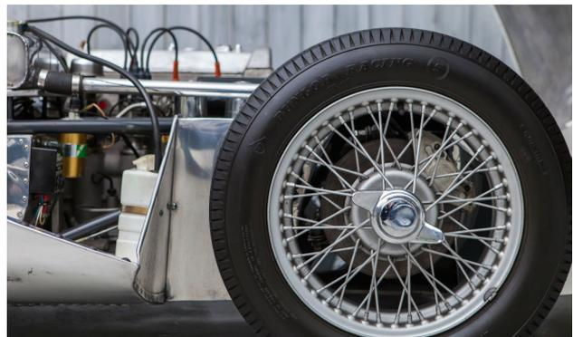
The Lotus 11 was a success from the start. With its lightweight multi-tubular space-frame chassis, stiffened by riveted stressed aluminium panels, it optimised all of Chapman's ethos for design - a lightweight chassis coupled with the latest in aerodynamic theory, engine, suspension and brake technologies. The frame alone weighed just 70lbs. Mostly powered by either the Coventry Climax 1,098cc FWA or 1,500cc FWB, they had an impressive power to weight ratio.
